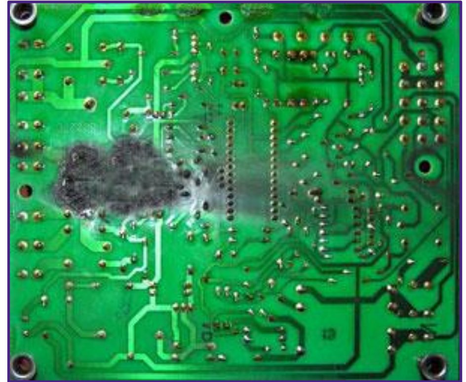
b) A burnt-out circuit board
